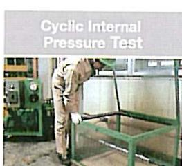
Cyclic pressure is applied 10,000 times. No leaks or problems were noted. / 注入 10,000 倍循环压力。没有发现泄漏或问题。/ Tekanan berkitar dikenakan sebanyak 10,000 kali. Tiada kebocoran atau masalah dikesan.
